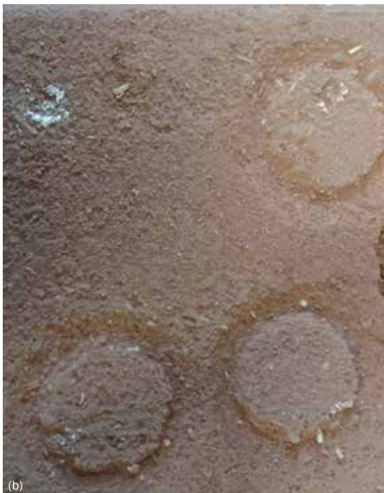
Figure 3. Specimens on brick of (a) CS30FS15_PCM30 mortar with cracking and (b) CS30FS45+F5 mortar after dry abrasion test.
